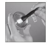
Reattach the shaver head and fit the distance ring. Use the brush for cleaning only. No need add water or oil to help. If necessary, wipe off the unit casing with a slightly dampened cloth.
