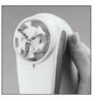
Brush out residual fuzz with cleaning brush provided. CAUTION: Blades are extremely sharp and can be damaged easily.
