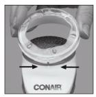
**TO FIT:** Push the distance ring onto the unit so that the recess on the distance ring engages the lug on the body of the shaver. This ensures that the distance ring does not twist when you adjust it.
